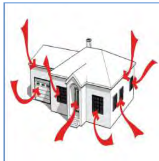
Figure 3 Voluntary Sound Insulation Program How Noise Enters a Home
